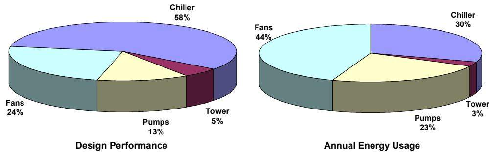
The series counterflow arrangement has improved the chiller performance as described in the sidebar. This has resulted in an overall design condition performance improvement.
