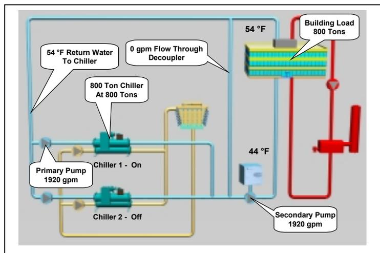
At full load, the design flow of 1920 gpm passes through the chiller, the two pumps, the load, and back to the chiller. There is no flow through the common pipe. At first, it would appear that the flow is being pumped twice. Although this is true, the total head is *split* between the two pumps. The primary pump is only sized for the primary loop of which the chiller is the main pressure drop. The secondary pump is sized for the pressure drop “outside the mechanical
