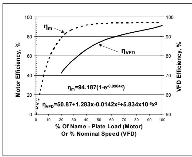
When both motors and VFDs operate at less than 100% capacity, their efficiency drops off. Figure 14 shows motor and VFD efficiencies at part load. It can be seen that oversizing motors can lead to significantly poorer performance than expected.
