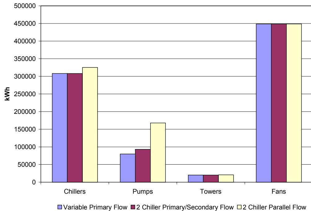
The parallel chiller constant flow arrangement can be used as a benchmark. Both the variable primary flow and primary/secondary flow arrangements have better chiller performance because the chillers can be staged off when not required.
