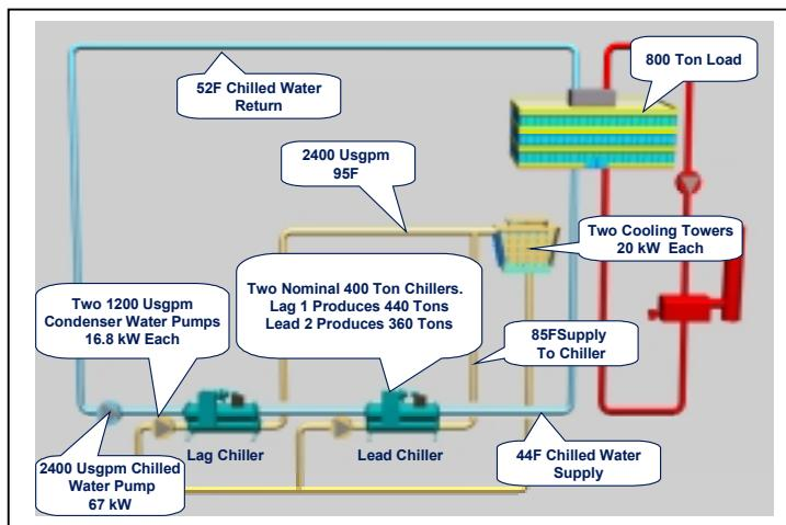
A problem with series chillers is the high flow rate and the low temperature range through the chillers. The high flow rate can result in high water pressure drops. Since the chillers are in series, the pressure drops of the chillers must be added. If the typical 10°F system temperature difference is maintained, then single pass evaporators should be considered. This will lower the pressure drop to an acceptable level.
