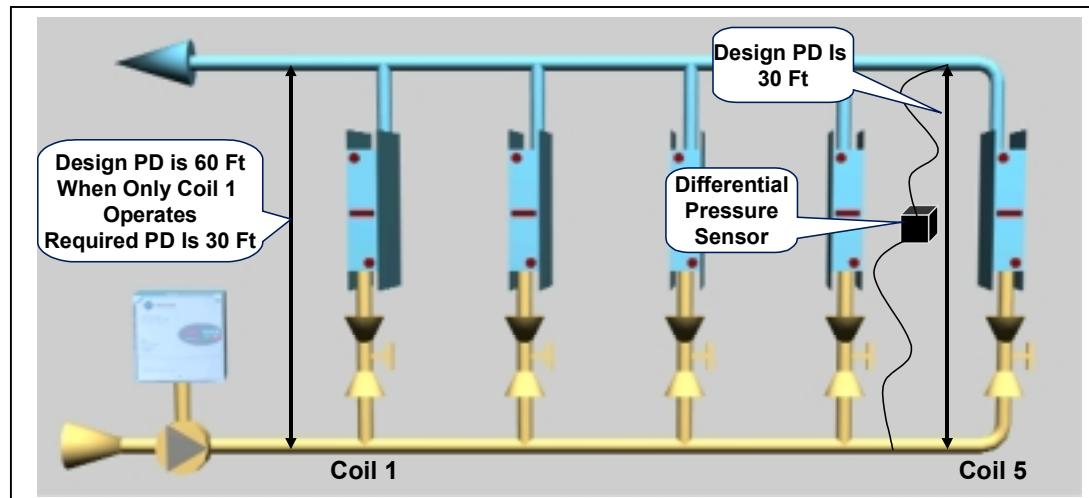
Another method of controlling variable flow pumps is to monitor the valve positions of a control valve in a critical part of the system. This valve is typically the furthest from the pumps. The control
