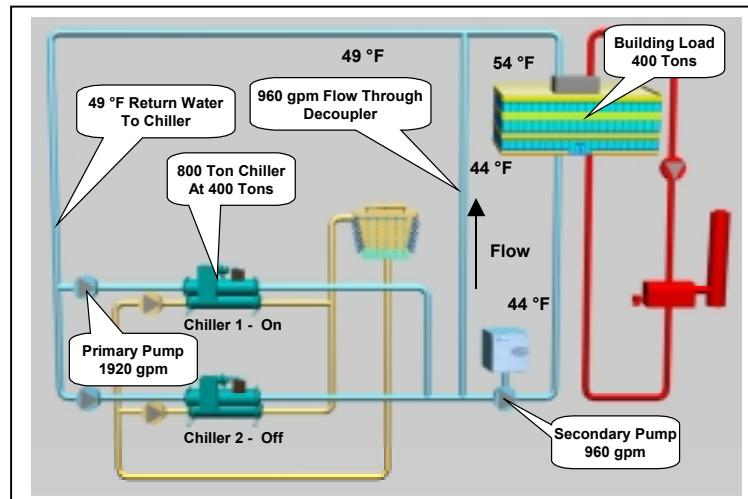
At full load, the design flow of 1920 gpm passes through the chiller, the two pumps, the load, and back to the chiller. There is no flow through the common pipe. At first, it would appear that the flow is being pumped twice. Although this is true, the total head is *split* between the two pumps. The primary pump is only sized for the primary loop of which the chiller is the main pressure drop. The secondary pump is sized for the pressure drop "outside" the mechanical room.
