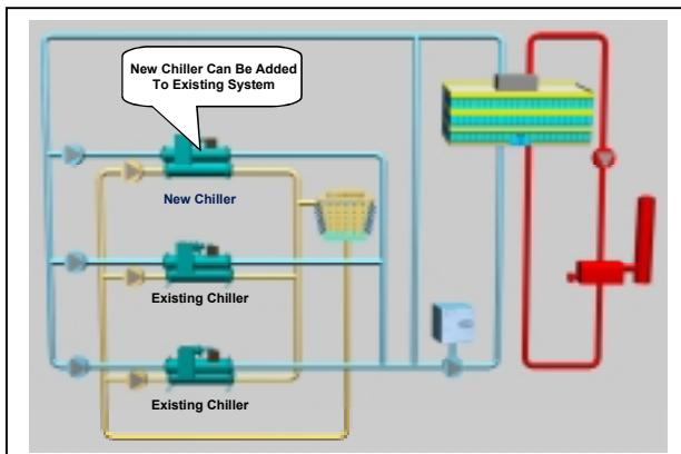
Primary/secondary piping allows easy expansion both in the chiller plant (primary loop) and the building (secondary loop). To expand the chiller plant capacity, another chiller can be added to the loop as shown in Figure 51. By strategically locating the decoupler and the new chiller (see Figure 49), it is possible to apply a greater load on the new chiller. This can be advantageous if the new chiller is more efficient than the rest of the plant.
