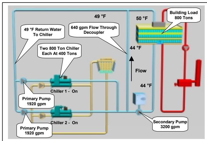
the primary pump horsepower. Finally, two chillers are operating (and their condenser water pumps) when only one should be.
