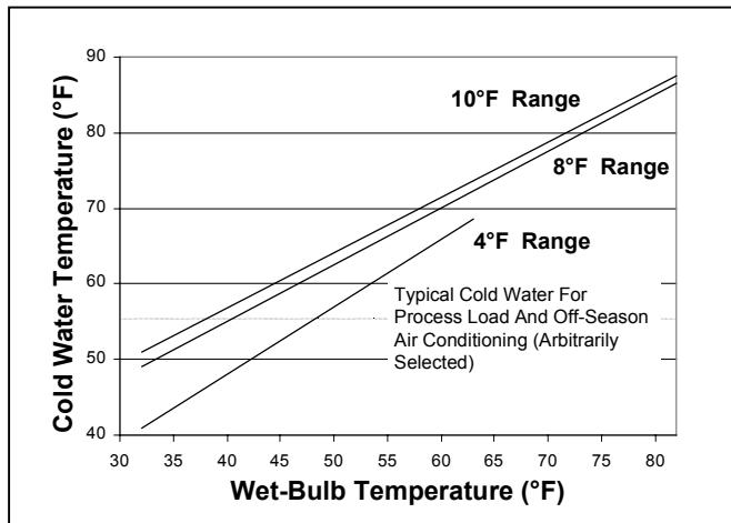
**Figure 58 - Cooling Tower Performance Optimized For Free Cooling**
