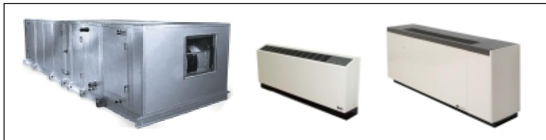
Chilled water coils are used to transfer the heat from the building air to the chilled water. The coils can be located in air handling units, fan coils, induction units, etc. The air is cooled and dehumidified as it passes through the coils. The chilled water temperature rises during the process.
