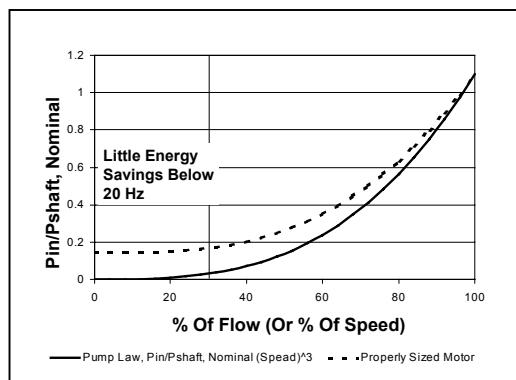
Figure 13 shows percent pumping power as a function of percent flow. From this figure, it can be seen that VFD pumps will not save much energy below 33% or 20Hz. Operating pumps much below 30% starts to create problems for motors, chiller minimum flows, etc. Since there are minimal savings anyway, the recommended minimum frequency is 20 Hz.
