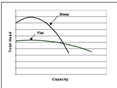
Figure 10 shows a steep and flat curve profile. Different pumps provide different profiles each with their own advantages. The steep curve is better suited for open systems such as cooling towers where high lift and stable flow are desirable. The flat profile is better suited for systems with control valves. The flat profile will maintain the necessary head over a wide flow range.
