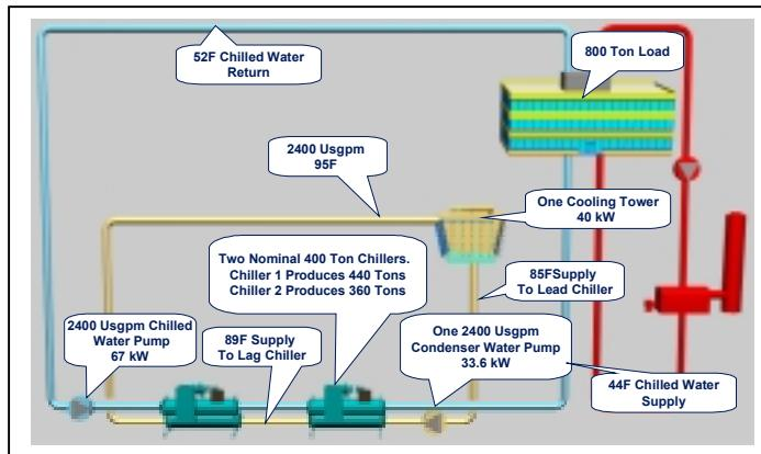
Series counter flow chillers can be 5 to 7% more efficient than a single chiller at design conditions and save up to 20% of chiller energy annually. However, the condenser pump is sized for the entire system flow (in this case 2400 US gpm) and this pump must operate whenever any chiller operates. The result is increased pump work annually. Series chillers with parallel towers may out perform series counterflow
