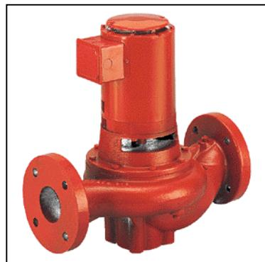
Typically centrifugal type pumps are used for both condenser water and chilled water systems. They can be either inline or base mounted. The pumps must be sized to maintain the system dynamic head and the required flow rate. Normally, the pumps are located so they discharge into the chiller heat exchangers.
