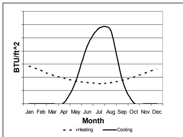
In many cases the cooling load is declining as the heat load is increasing. An example is reheat for VAV. Without a cooling load, no heat can be collected. An analysis must be performed to identify the size and time of heating load. McQuay Energy Analyzer™ can perform the analysis and recommend heat recovery, Templifier™ and source chiller sizing. Then the cooling load at the same time periods must be identified. Some or all of the heat from the cooling load can be used for the heating load.
