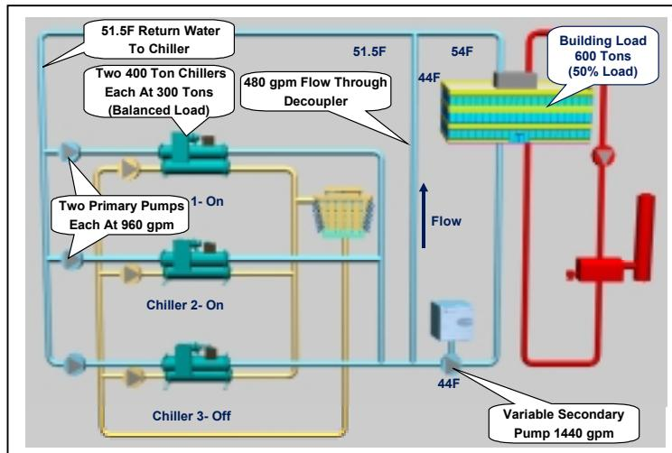
Figure 42 shows a 1200-ton primary secondary system with three chillers. The system is operating at 50% or 600 tons. The 600-ton load requires 1440 gpm. Two chillers are operating along with their 960 gpm primary pumps.
