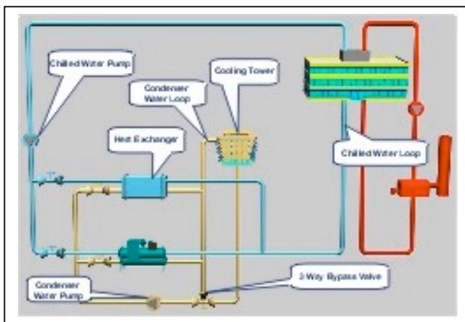
This system is “non-integrated” meaning it can only be either mechanical cooling or free cooling. Nonintegrated systems generally do not offer as much savings as integrated systems but avoid additional operating hours for chillers at light loads. Continuous light load operation for some chillers can lead to operational difficulties such as oil migration or repeated starts.
