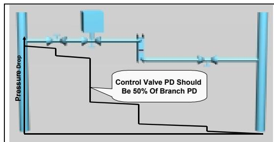
Figure 22 shows typical pressure drops from the supply to the return line for a cooling coil. For a modulating valve, the valve pressure drop should be as large a percentage as possible when compared to the system pressure drop; preferably over 50%. The reason is to maintain valve authority. For on-off control, any valve can be used as long as it can pass the required flow rate with the pressure differential available.
