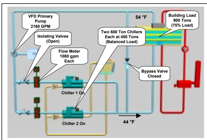
Variable primary flow provides pump savings over primary secondary systems because all the chilled water being pumped is being used for cooling. In a primary /secondary system, any flow through the decoupler consumes pump power but provides no cooling.
