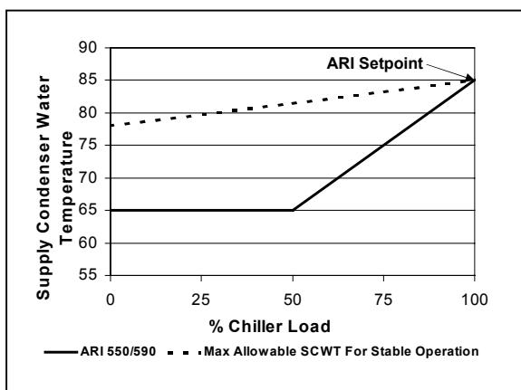
If aquastats are going to be used, then a lower setpoint than 85°F should be used. One recommendation is to set the aquastat at the minimum condenser water temperature acceptable to the chiller. The cooling tower will then operate at maximum fan power and always provide the coldest possible (based on load and ambient wet bulb) condenser water to the chiller until the minimum setpoint is reached. Then the tower fan work will stage down and maintain minimum setpoint.
