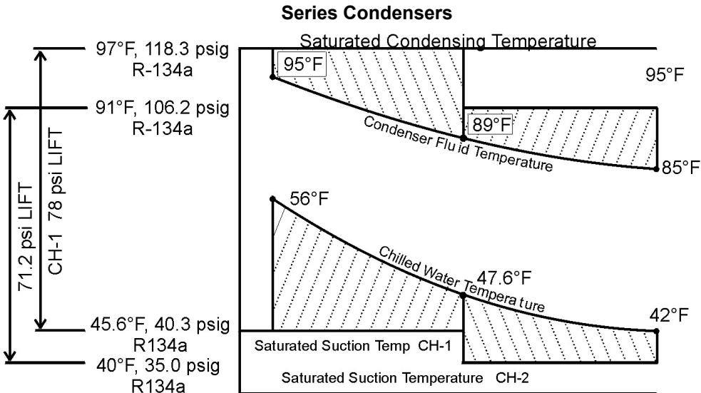
The above figure shows the lift requirements for series counterflow chillers. Now chiller-2 sees a lower lift because the discharge pressure has been reduced as a result of the lower condenser water temperatures. The chiller lifts are almost balanced which will always provide the best refrigeration performance.
