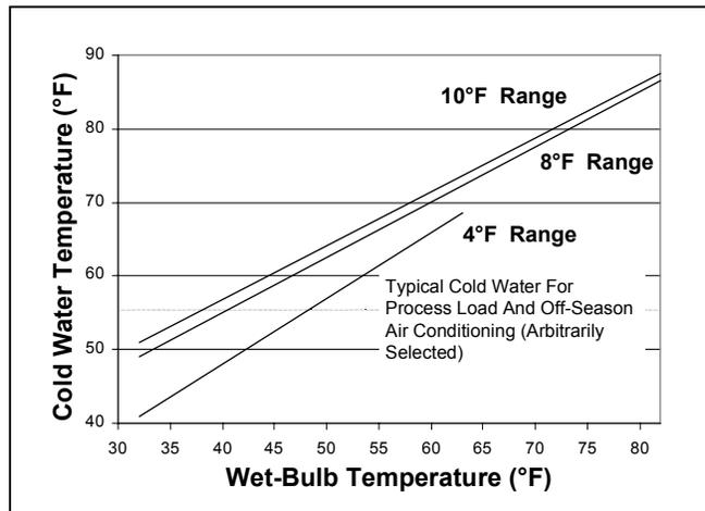
**Figure 58 - Cooling Tower Performance Optimized For Free Cooling**
