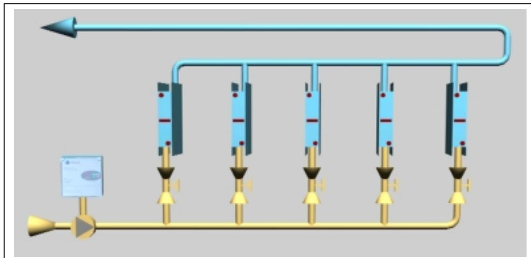
Figure 6 shows reverse return piping. Reverse return piping is designed such that the path through any load is the same length and therefore has approximately the same fluid pressure drop. Reverse return piping is inherently self-balancing. It also requires more piping and consequently is more expensive.
