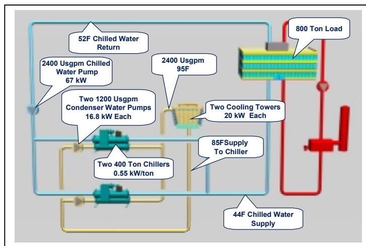
For constant flow systems, the chilled water temperature range varies directly with the load. Depending on load diversity, the chiller design temperature range will be less than the temperature range seen at each load. In this case, the chiller temperature range is 8°F while the cooling coil range is 10°F (Refer to **Piping Diversity**, page 24). The overall result is increased chilled water pump and pipe capital cost plus higher annual pumping cost.
