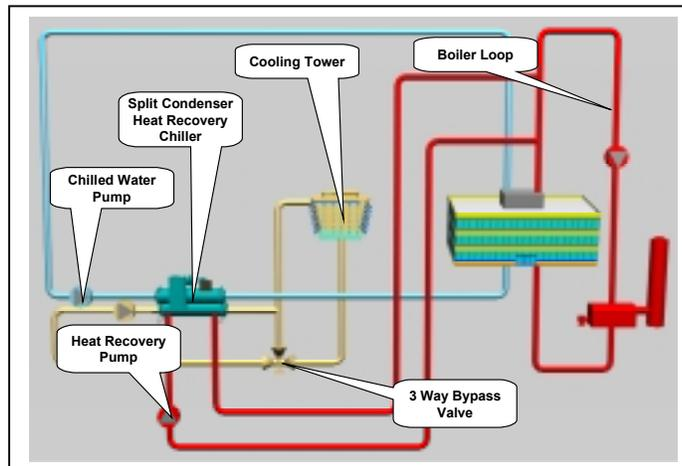
Figure 62 shows the piping arrangement for a split type heat recovery chiller. The hot water loop flows directly through the chiller. Any additional heat not used by the hot water loop is collected in the condenser loop and rejected by the cooling tower.
