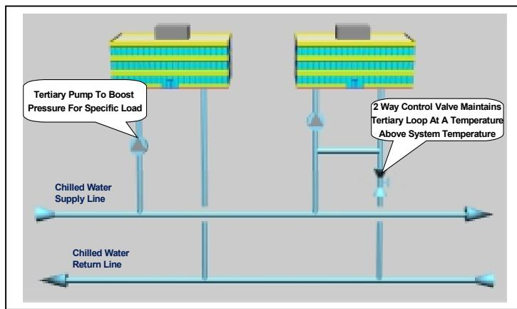
load is greater than the pressure differential available in the main secondary loop. This often happens when a new load is added to an existing loop. An additional tertiary pump is added to provide additional pressure to overcome the specific load.
