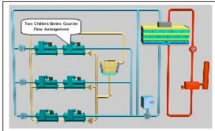
Figure 52 shows series counterflow chillers in a primary/secondary system. The series counterflow arrangement provides an efficient means to produce 40°F supply water with an 18°F temperature range. The series counterflow arrangement can provide about 5% better annual performance than single large chillers when using large temperature ranges.
