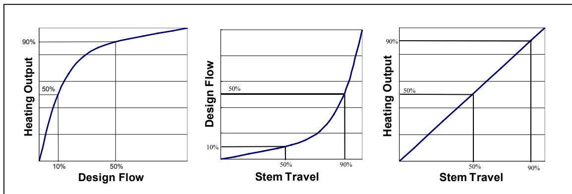
**Figure 21 - Coil and Control Valve Performance Curves**
