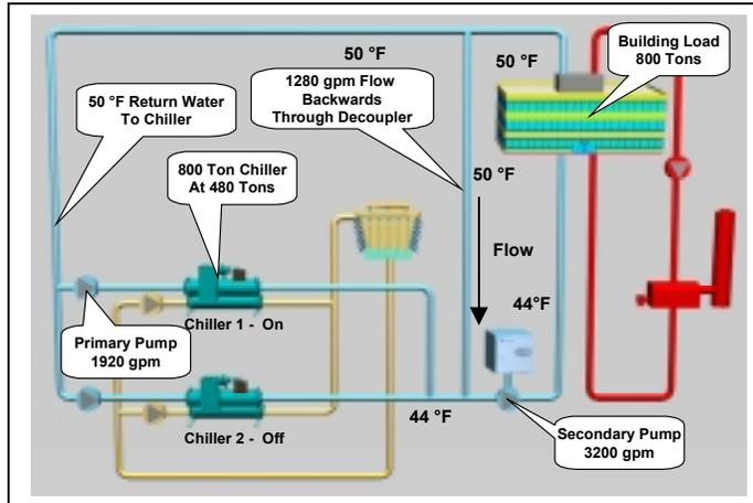
It is important to understand what happens if design temperature range is not maintained. This is known as a low delta T syndrome. Figure 70 shows the previous example with an 800 ton load but only a 6°F delta T. This could be caused by several factors including poor valve selection or dirty coils.
