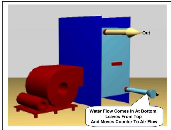
Coils must be connected so the water flow through the rows of the coil is counterflow to the airflow. When coils are improperly connected, the coil performance can drop by as much as 15%. When this occurs, the chilled water control valve will go wide open because the coil is in effect, 15% undersized.
