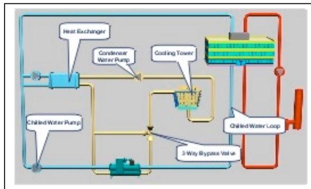
Figure 56 shows a modified version where the heat exchanger uses a small tertiary loop and a dedicated pump. This arrangement removes the heat exchanger pressure drop from the main chilled water system.
