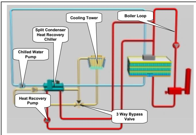
Figure 62 shows the piping arrangement for a split type heat recovery chiller. The hot water loop flows directly through the chiller. Any additional heat not used by the hot water loop is collected in the condenser loop and rejected by the cooling tower.
