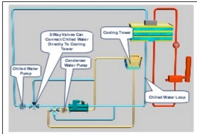
There are several ways to provide waterside free cooling. The chilled water loop can be connected by means of three-way valves, directly to the cooling tower in a “strainer cycle” method. This method is not preferred because the chilled water loop is then exposed to atmosphere introducing dirt and creating water treatment difficulties.
