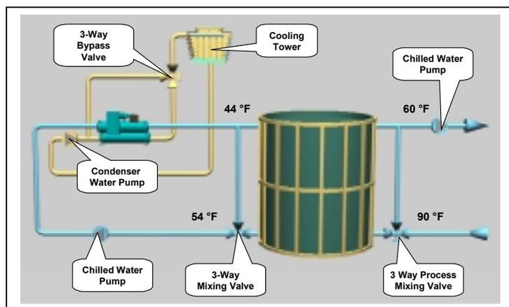
Figure 75 shows a typical piping arrangement to deal with high supply water temperature, large temperature range and small chilled water volume.
