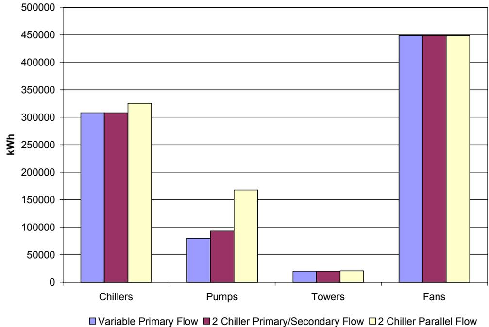
The parallel chiller constant flow arrangement can be used as a benchmark. Both the variable primary flow and primary/secondary flow arrangements have better chiller performance because the chillers can be stage off when not required.
