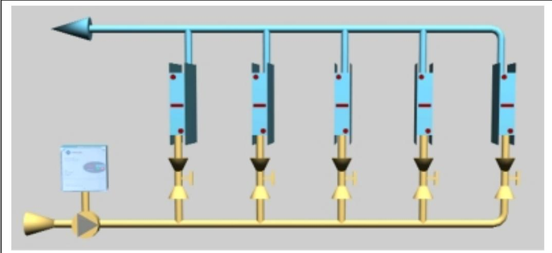
Direct return piping results in the load closest to the chiller plant having the shortest path and therefore the lowest fluid pressure drop. Depending on the piping design, the difference in pressure drops between a load near the chiller plant and a load at the end of the piping run can be substantial. Balancing valves will be required. The advantage of direct return piping is the cost savings of less piping.
