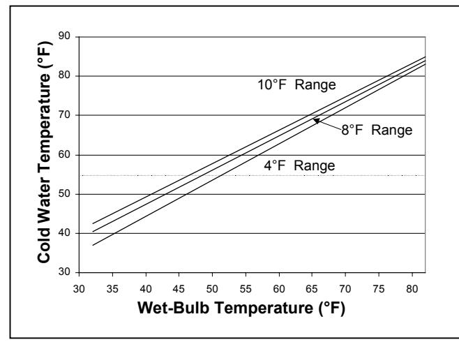
Figure 58 shows a cooling tower optimized for free cooling. The cooling tower was selected to provide 48°F condenser water at a 45°F wetbulb and 4°F range (50% building load). This allows 50°F chilled water to be produced.
