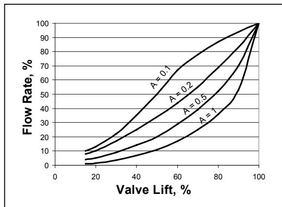
Figure 23 shows the change in the valve characteristic that occurs at different Valve Authorities. Since the goal is to provide a valve with a performance characteristic that is the opposite of a coil characteristic (See Figure 21), it is important to maintain Valve Authority above 0.5.
