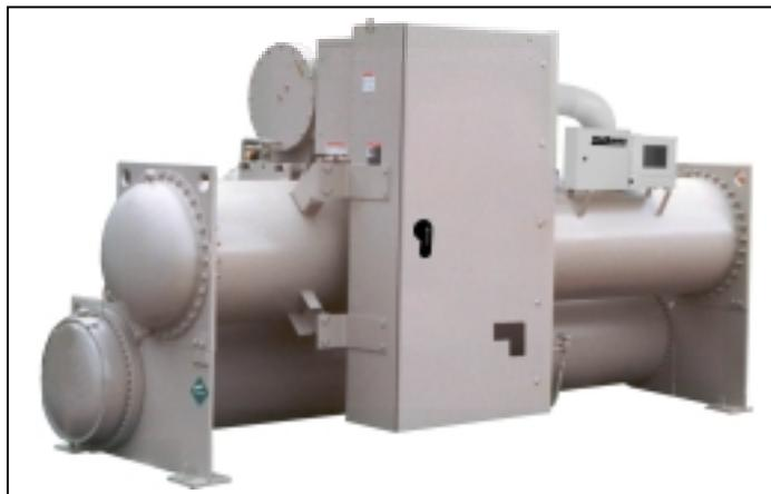
The best way to take advantage of a VFD chiller is to reduce the condenser water temperature as much as possible. Climates with reasonable annual changes in wetbulb are prime candidates for VFD chillers.
