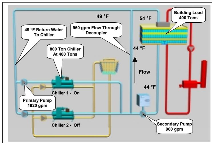
Figure 69 shows the same example operating at 50% capacity. The two-way control valve at the load has reduced the flow in the secondary loop to 960 gpm. The delta T across the load remains at 10°F.
