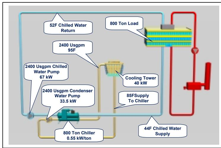
For constant flow systems, the chilled water temperature range varies directly with the load. Depending on the load diversity, the chiller design temperature range will be less than the range seen at each load. In this case, the chiller range is 8°F while the cooling coil range is 10°F (Refer to **Piping Diversity**, page 24). The overall result is increased chilled water pump and pipe capital cost plus higher annual pumping cost.
