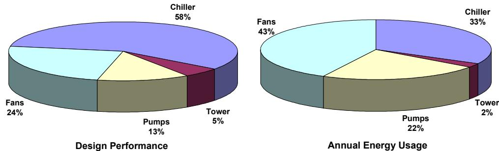
The design load performance is identical to the single chiller plant. There are small changes in real applications when two chillers are used instead of one. For instance, pump and chiller selections are not likely to offer identical performance, other than being half the size.
