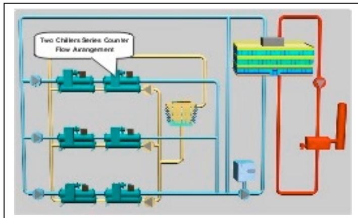
Figure 52 shows series counterflow chillers in a primary/secondary system. The series counterflow arrangement provides an efficient means to produce 40°F supply water with 18°F temperature range. The series counterflow arrangement can provide about 5% better annual performance than single large chillers when using large temperature ranges.
