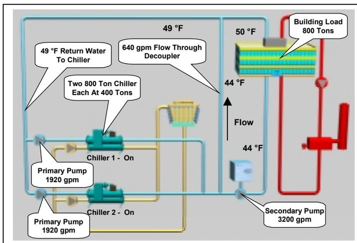
Obviously the above example can’t occur. Figure 71 shows what does happen. A second chiller has to be started to balance the flow in the primary loop with the flow in the secondary loop.
