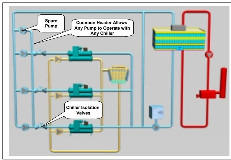
The flow for each chiller is based on the design flow required by the chiller. The flow is only provided when the chiller is operating. An automatic isolating valve is required for each chiller to stop short-circuiting when the chiller and pump are off.
