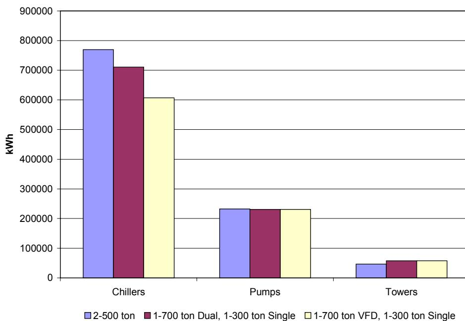
The two 500-ton chillers provide a benchmark. Since the hospital has a load profile with many hours between 50 and 70% of design capacity, the next two options outperform the benchmark. During these hours, only one chiller is required to meet the load avoiding the need for two primary and condenser pumps. The result is more efficient use of the chiller and reduced pump work.
